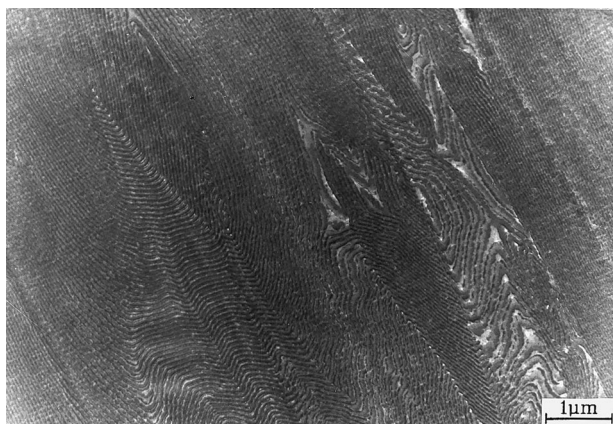
Fig. 5. TEM micrograph of sample SBM270 with lamellar structures ( \Phi_{\text{PS}} = 0.70 , M_n = 270 kg/mol) where the microphases are intermediately segregated.
